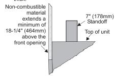
Install Top Standoffs & Side Nailing Strips before unit is slipped into position. See the "Unit Assembly Prior to Installation" section for assembly details.
